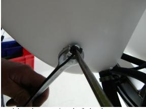
...and drop the sensor into the fuel tank.
