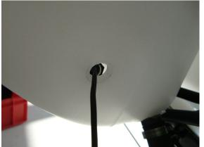
Remove the sensor with the rubber washer from the fuel tank through the filler neck with a wire.
